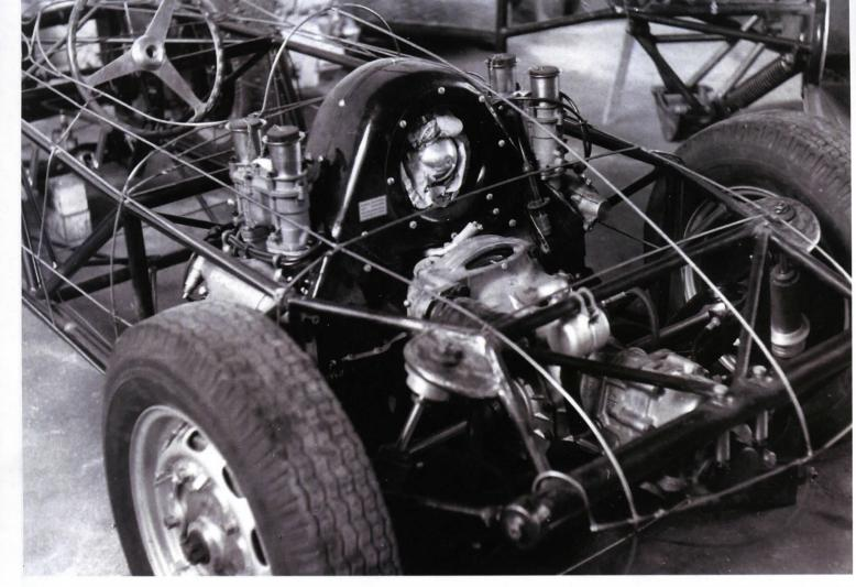
trailing wishbones at the rear of the single-seater that Porsche was building, Colotti made a good fist of it. In fact he put the coil/damper mounting platforms outside the frame instead of inside so that the main tubular structure could be narrower for strength and better body lines.
